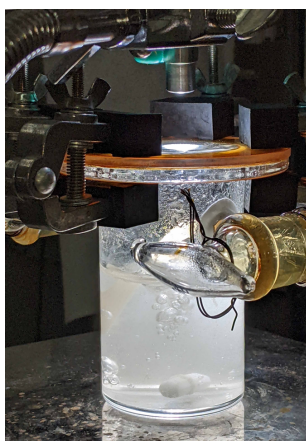
Chart S2. Photocatalytic Pyrex Flask Reactors Containing H 2 O (70 mL) Equipped with Quartz Window on the Top Irradiated with UV–Visible Light from a 300 W Xe Arc Lamp through a Quartz Light Guide. Light intensity 222 mW per flask.
